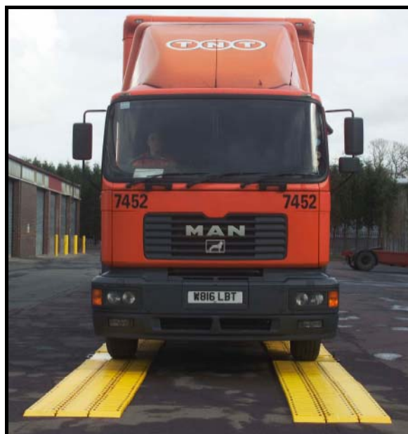
Figure 5.2.1.3 Surface mounted weigh pads with infill strips
