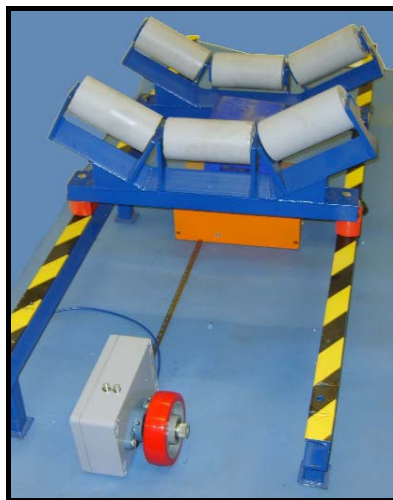
Figure 5.1.1.2 Belt weigher with two idler weighing mechanism
