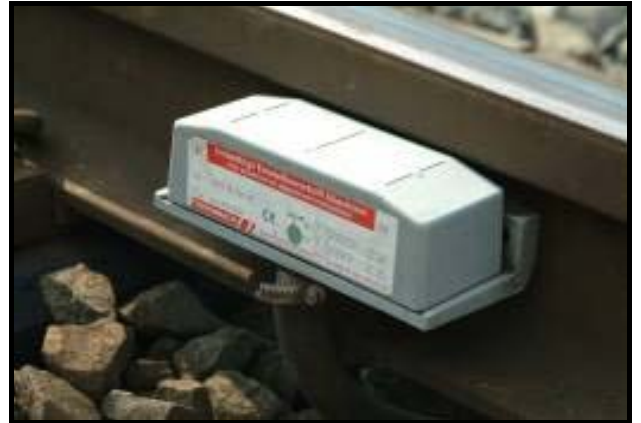
Figure 5.2.2.2 Inductive sensor wheel detector
